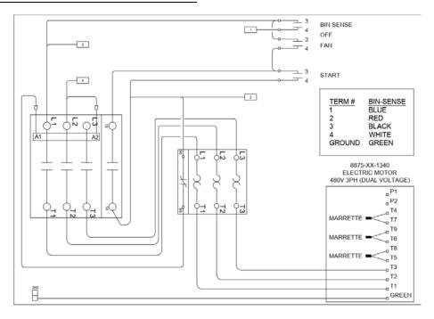
15.15 3HP, 5HP, 7.5HP Inline & Turbo Centrifugal Fan 10HP & 15HP Inline Centrifugal Fan (600V, 3PH)
